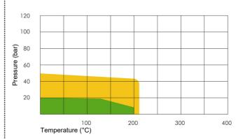
The P x T diagram above indicates the service limits for **NA-1006** considering the simultaneous influence of pressure and temperature (chemical suitability assumed). The green area represents the normal service limits, while the orange colored area shows the maximum application limits. For those cases, please consult our technical department.
